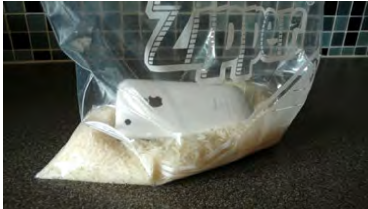
Figure 1.1: My wife's wet iPhone in a plastic bag with rice for dehumidification
