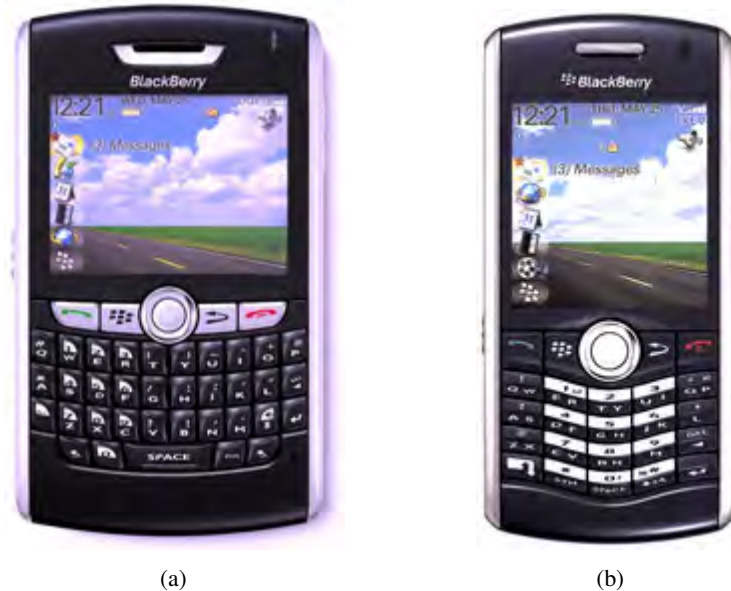
Figure 6.1: (a) BlackBerry 8800 with larger screen and QWERTY keyboard; (b) BlackBerry 8100 Pearl with smaller screen and SureType keyboard
